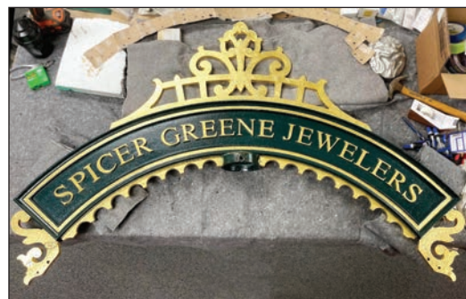
Restored 1920 Seth Thomas No.2 cast iron sign ornament. Powder-coated, gold-leafed with raised aluminum letters.
