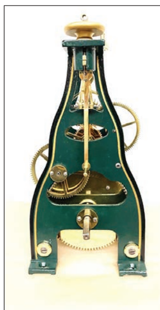
Restored 1910 E Howard Street Clock Movement (front view)
