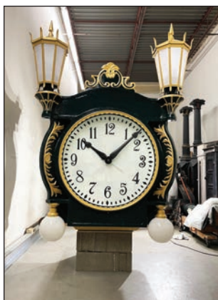
1911 Joseph Mayer "Tulip Top" base with "rhomboidal" eight lamp, four dial top. Restored four dial head with 42-inch dials
