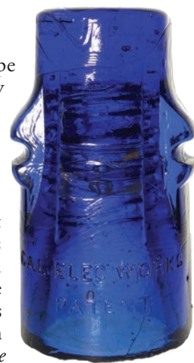
Cobalt blue glass insulator for California Electric Works (San Francisco)
