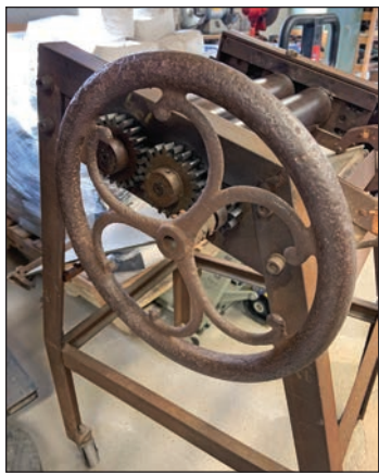
The “Roller Thing,” a hand-made tool used to press glass and “get the bubbles out” with an antique turning wheel pulled from the ground.
