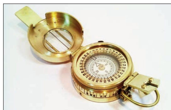
This brass compass dates back to World War II. The rose has 36 points on the outer rim with hundreds of other marks on the inner parts of the dial.
