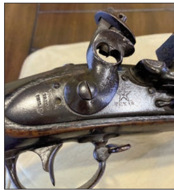
Correct "TEXAS" and star stamp forward of cock, contractor "TRYON / PHILADA" marking stamped vertically at the tail
