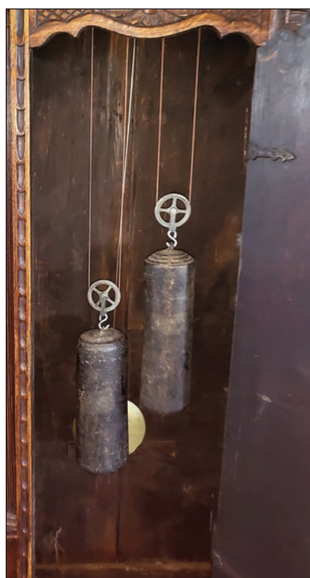
The lower door houses two iron weights, the pendulum, pendulum bob and time adjustment screw.
