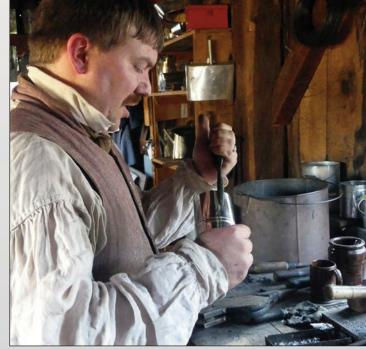
Many items such as this cup have a joint made by overlapping itself. This overlap is then soldered – which to hold it for soldering is held by a pair of pliers as to not burn the tin plate worker.
