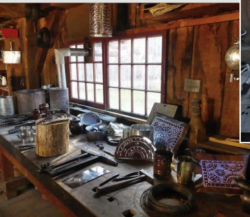
The tin plate worker's workbenches were constructed similarly to other workbenches in other trades. These would have square holes in them to hold such tools as the one laying on the bench called swages or stakes which are similar to anvils.
