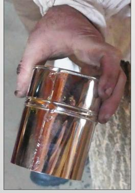
After soldering the cups body, the solder hardens, holding the cup together and making that section water-tight.
