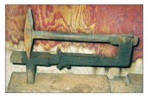
This style of anvil was called a "stake" anvil and was used by the tinsmith to create creases in the metal for a variety of small items. This tool is seen placed on top of a blacksmith's anvil. (photo: ebay)
