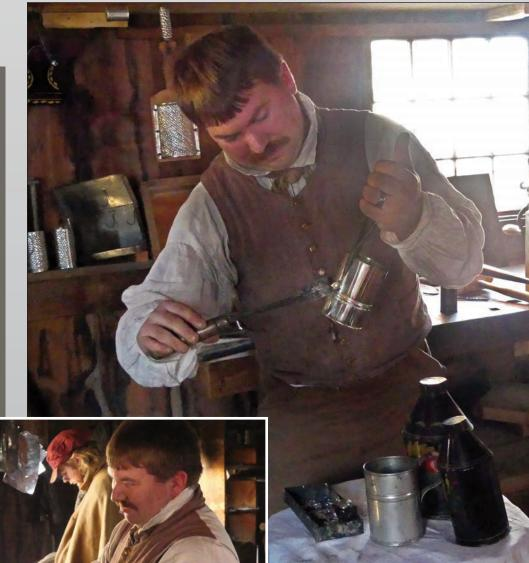
As a tinplate worker starts to solder the joint of the cup body he starts where the pliers are, and an angular soldering iron pulls the solder away letting the heat warm up the cup allowing the solder to flow and level out making the cup one piece.
