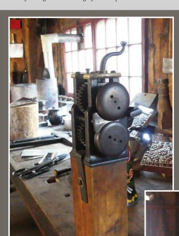
This wiring machine, ca. 1840s produced by Peck Smith & Co., is one of a full set of machines used to roll the edges to create different joints.
