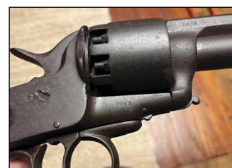
18 gauge shotgun barrel below .42 caliber rifled pistol barrel, 9 shot cylinder.
