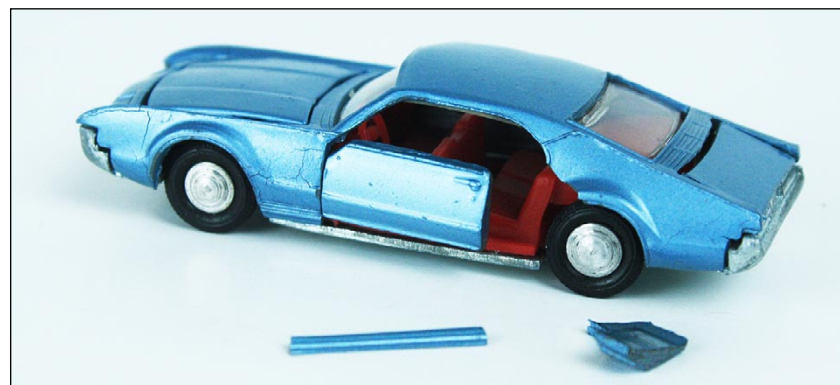
The baseplate on this Mini Dinky Oldsmobile has expanded and distorted, resulting in parts of the body breaking off.
