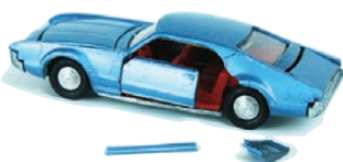
The baseplate on this Mini Dinky Oldsmobile has expanded and distorted, resulting in parts of the body breaking off.
