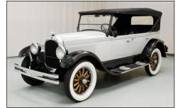
Introduced in 1924, the Chrysler Six boasted only 201 cubic inches but its 4.7:1 compression ratio engine delivered 68 horsepower. Chrysler was one of the first to adopt 4-wheel hydraulic brakes and the Chrysler Six also had full pressure engine lubrication. No wonder Chrysler sold 32,000 of them in its first year.
