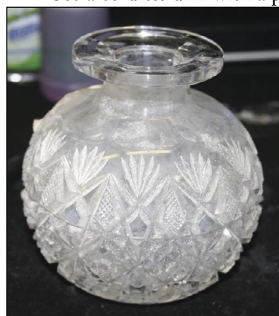
Cut glass clouded by a white film possibly damaged by detergents or chemicals
