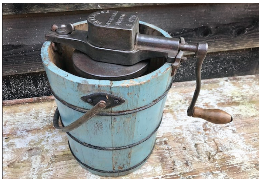
1920s Husqvarna Ice Cream Maker, complete with all the inner workings, but a great-looking piece in lovely blue paint. Ice and some salt were placed in the outer rim of the bucket, and ice cream mixture went in the inner chamber. Turning the handle paddles the ice cream, churning and freezing it simultaneously.
