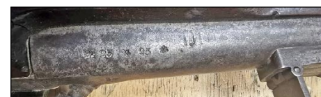
The barrel proofs "25" and "25" show that the barrel was gauged after boring and after test firing. 25 bore translated to .577 caliber.
